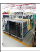
Parts trolley, with PU Coated pipes
