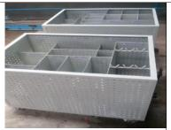
Exhaust Pipe Trolley for Odd Shape pipes
