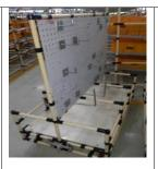
Hooks are attached on the Trolley as per components
