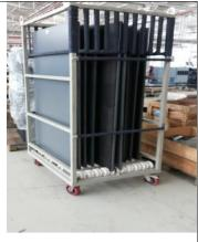
Truck mountable Trolleys for transportation Powder Coated Parts. (Green color PVC Coated pipes, Frp sheets, Rubber bushes are used to avoid metal to metal contact)
